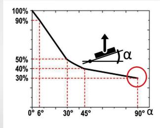
**Maximum load weight with 3:1 safety factor = 90 kg x 100 % x 30 % = 27 kg**
